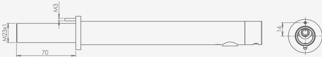
4. Insert the faucet and its attachments through the wall. The aerator in the faucet spout must face the washbasin.
